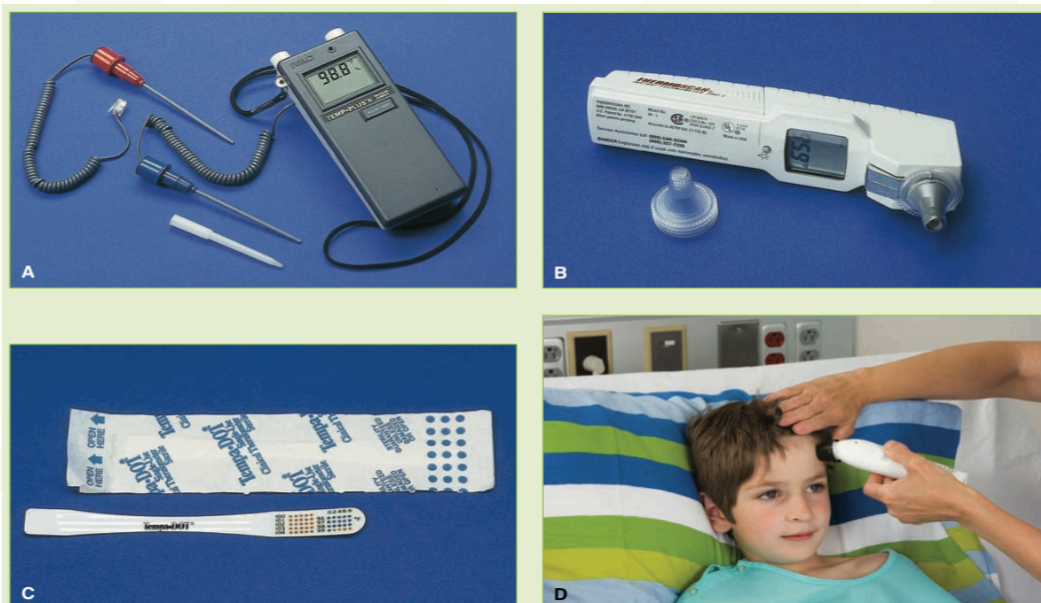
FIGURE 1. Types of thermometers. (A) Electronic thermometer. (B) Tympanic membrane thermometer. (C) Disposable paper thermometer; the dots change color to indicate temperature. (D) Temporal artery thermometer.
